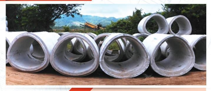
**Tubo TechSpan®** is a prefabricated reinforced concrete tube with vaulted sections that has particular designs for small cross structures like road sewers, culverts, any other utility pass, etc. To install the **Tubo TechSpan®**, a trench is excavated at the installation location as per the dimensions of the Tubo TechSpan®. Waterproof structures can be built using these segmental units.
