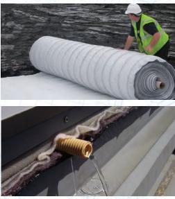
DRAINTUBE<sup>™</sup> has unique benefits over other geocomposite drainage systems; such as no geotextile intrusion, no creep and no peel adhesion issue. These ensure long term performance in most difficult conditions. Each roll performs the functions of separation, filtration and drainage.
