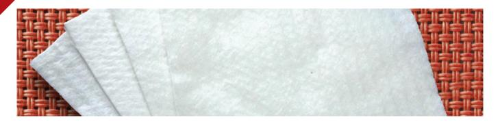
TerraTextile - W  $\mathrm{Mu_{pp}}$  are woven geotextiles manufactured from high strength polypropylene multifilament yarns that are woven together to form a dimensionally stable and highly permeable fabric structure. This type of TerraTextile fabrics have superior resistance to soil and biological clogging and acts efficiently as filter. This type of TerraTextile behaves very well as separator and stabiliser, allowing water to freely pass through while preventing soil erosion.
