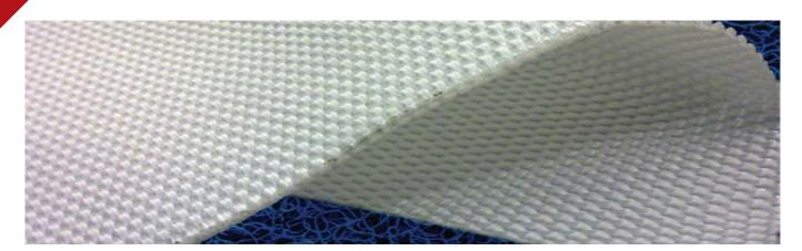
TerraTextile – W  $\mathrm{Mu}_{\mathrm{PET}}$  are woven geotextiles with individual threads (multifilaments) of polyester yarns that are woven together on a loom to form a stable fabric structure. This type of woven TerraTextile fabric display superior mechanical and hydraulic properties along with excellent resistance to biological and chemical environments normally found in soils.
