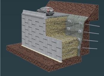
TerraLink<sup>®</sup> allows building new Reinforced Earth type walls connected to retaining structures such as slopes stabilized by nailing or existing retaining wall.
